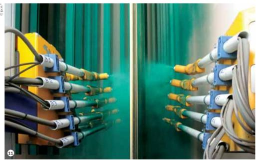
Figure 11: Two of the four groups of spraying guns.
