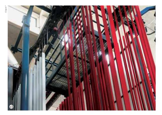
Figure 13: DFV work with a very high productivity: only few centimetres are left between two colours.
