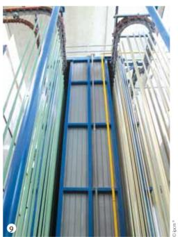
Figure 9: The curing oven.
