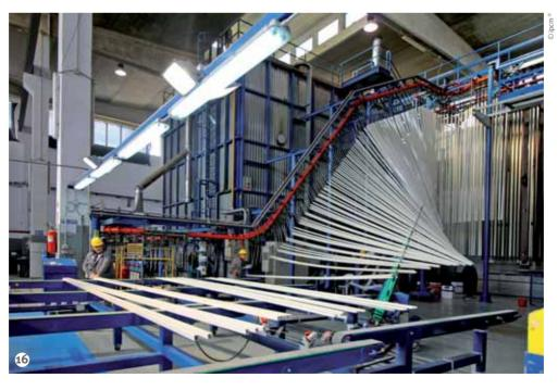
Figure 16: The unloading station.
