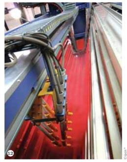
Figure 12: The inside of the coating booth.
