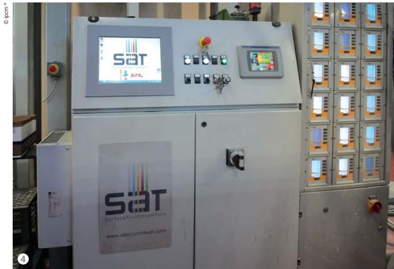
Figure 4: Sepal can manage both the booth and the guns with one control panel.
