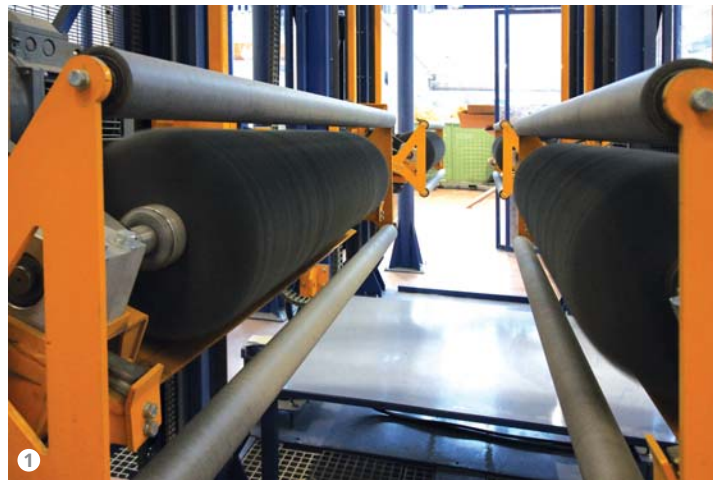
Figure 1: The brushes scratch the profiles' first layer of aluminium to significantly reduce the possibility that surface defects appear after coating.
