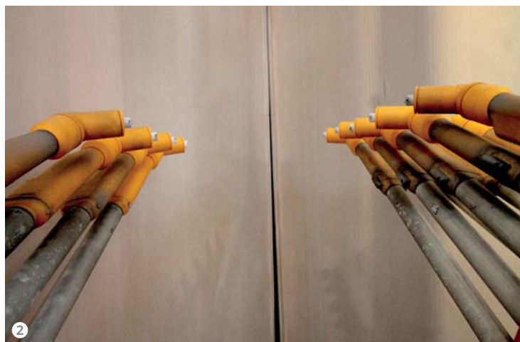
Figure 2: The coating booths feature 18 guns each.
