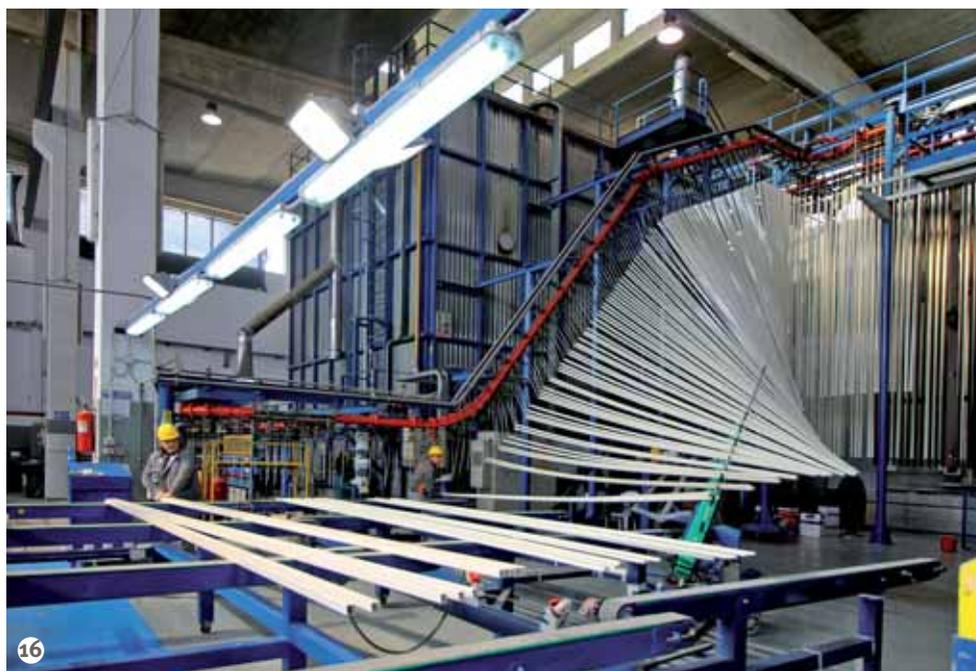
**Figure 16: The unloading station.**
