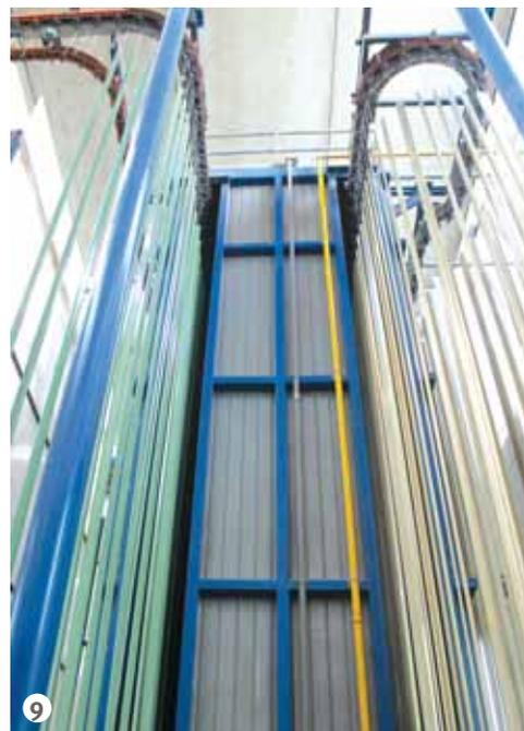
Figure 9: The curing oven.
