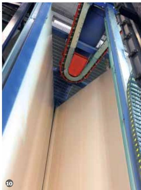
Figure 10: The “V” shaped coating booth.
