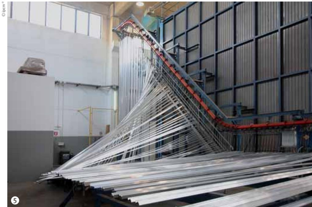
**Figure 5: The loading station.**
