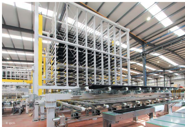
From top left clockwise: Powder application with Gema SIT technology; The powder centres of the two C-Expert booths; The automatic unloading system with five transport belts; Storage buffers housing the coated profiles to be sorted towards the assembly, packaging, and plasticisation lines.
