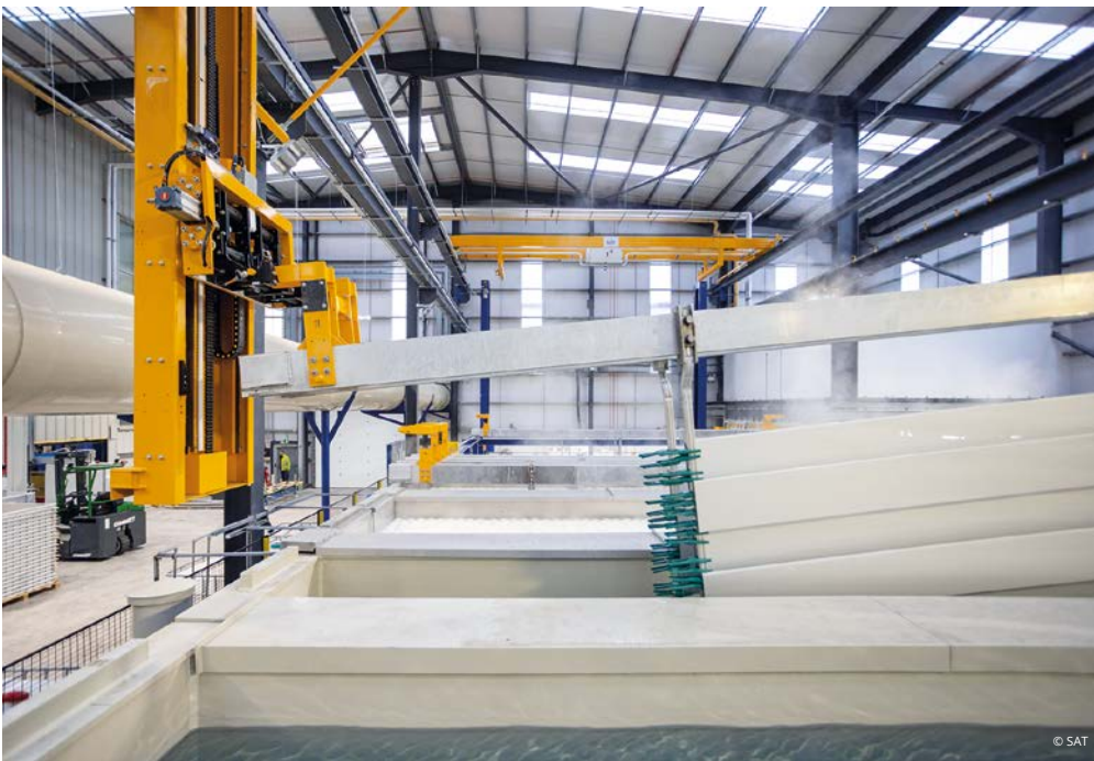
Each bridge crane has a device on board to adjust the distance between the two anodic bars.
