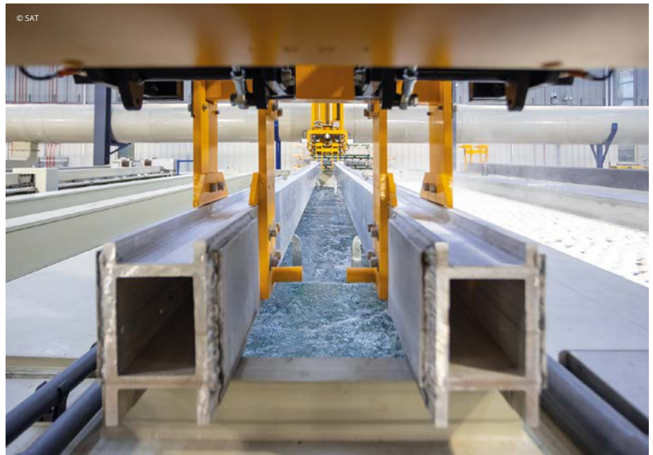
Immersion of the bars in a process tank.
